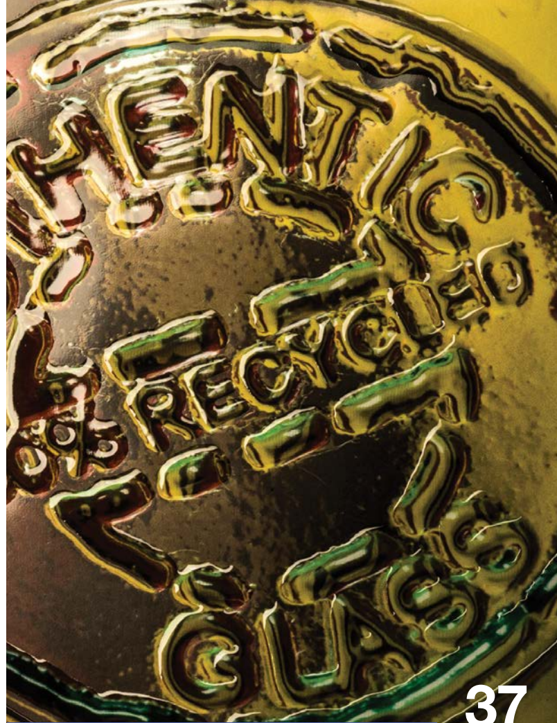
Picture shows a label printed using Xaar's High Laydown Technology
