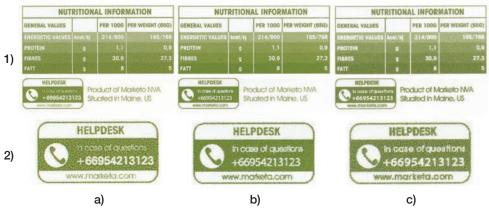
Figure 12: Identical images printed with effective addressability of: a) 600 dpi b) 360 dpi c) 720 dpi
