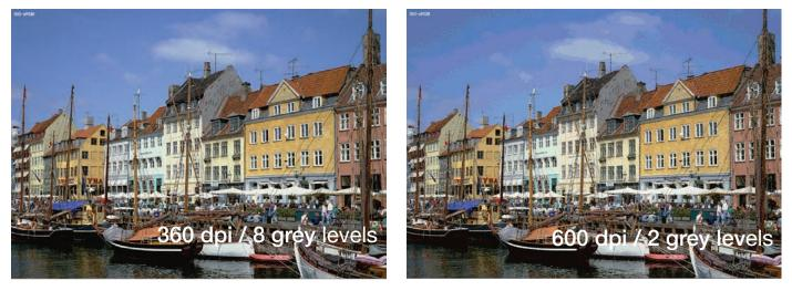
Figure 8: Digital image simulation of 360 dpi with 8 grey levels compared to 600 dpi with 2 grey levels
